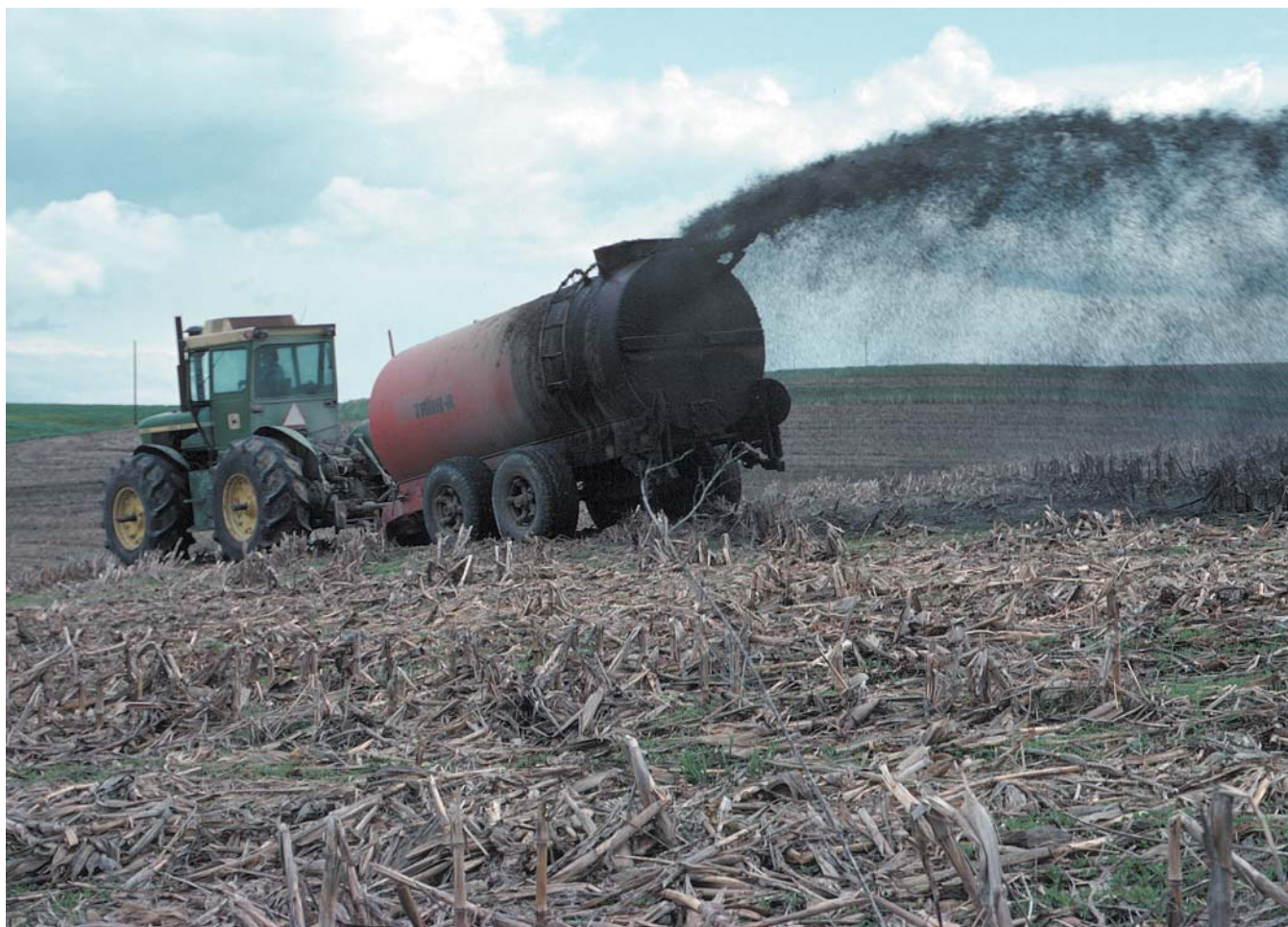
Liquids from anaerobic lagoons and other storage systems are distributed over cropland using "honey wagons". Photo Courtesy of USDA NRCS.
